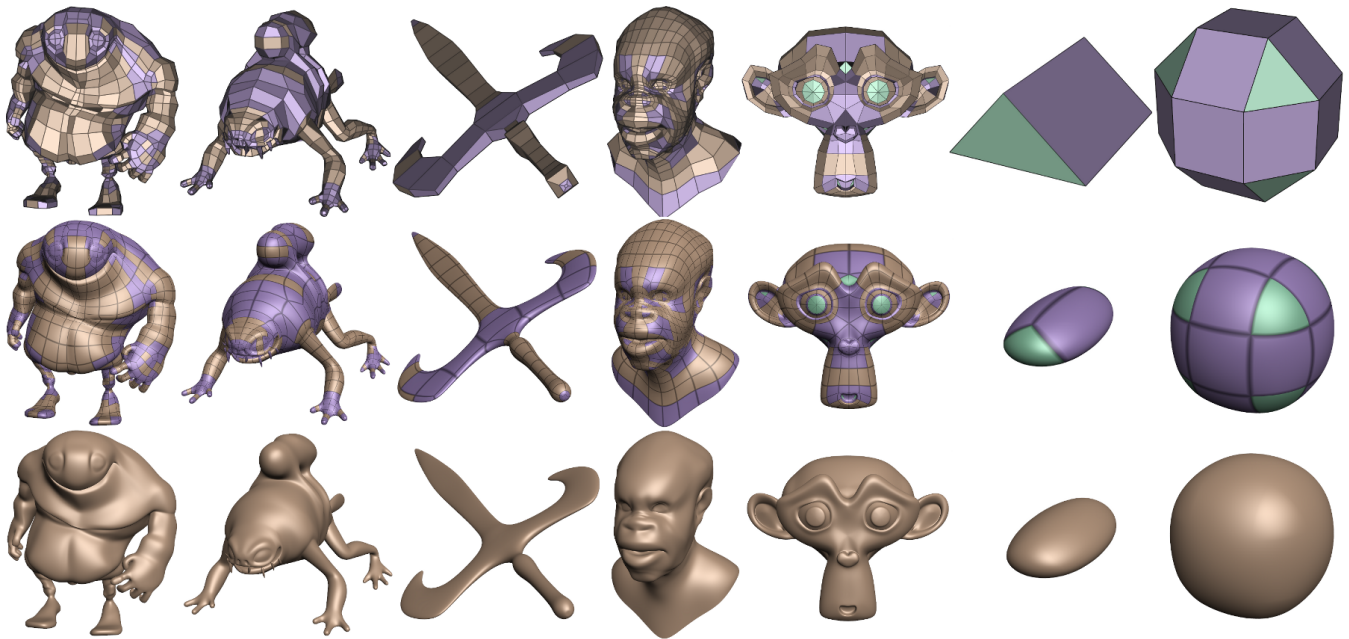
Figure 12: From top to bottom: the input mesh, the patch structure (regular patch in gold, irregular quad patch in purple, triangular patch in green), and our smooth surface. Columns 1-3 contain closed quadrilateral meshes. Column 4 is a quadrilateral mesh with boundary, and columns 5-7 contain closed tri/quad meshes.
