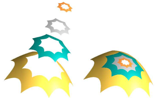
Figure 9: Subdivision surfaces consist of a nested sequence of surface rings.
